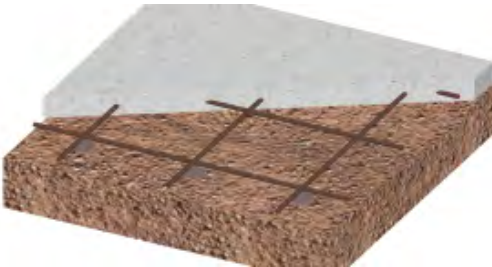
REINFORCEMENT_LIGHT BARS EACH WAY
